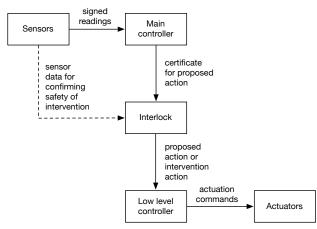
Figure 1: Certified control architecture
